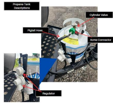
counterclockwise. Connections must be tight, however DO NOT overtighten.
