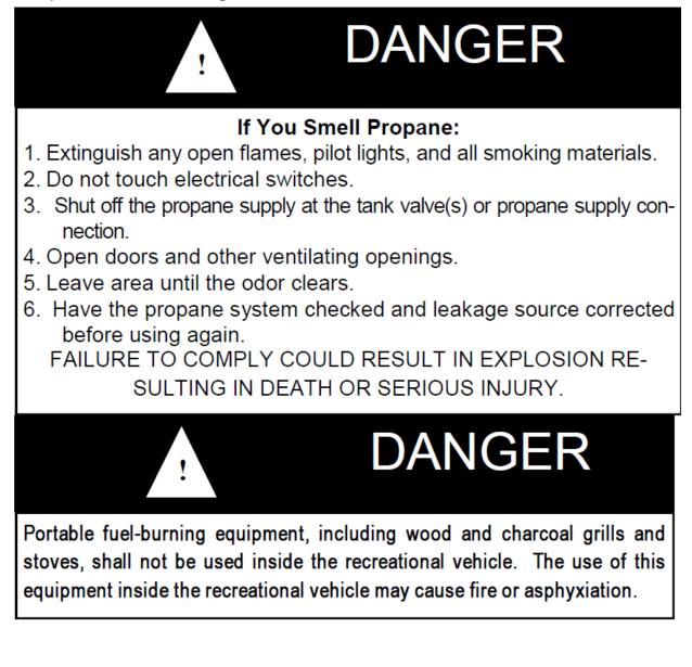
It is especially important that cooking appliances **not be used for comfort heating,** as the danger of asphyxiation and unsafe levels of carbon monoxide are greater when the appliance is used for long periods of time.
